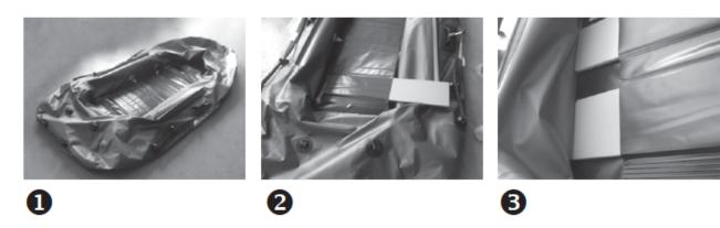
NOTE: Make perfectly sure that each floor board is well centred, as it will be difficult to reposition the board once the boat is fully inflated.
